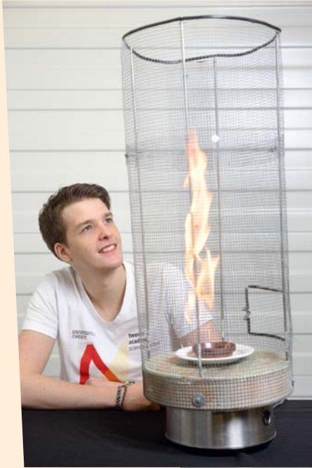
This fire tornado shows the effect of a vertical airflow, which is created by swirling the appliance around a small flame.
